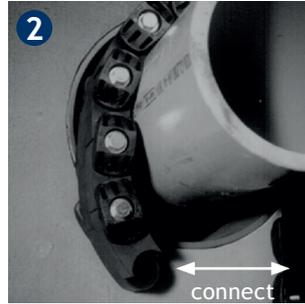
**2** Use only in suitable wall sleeves, installation tolerances according to dimensions in the calculation program. The specified clamping ranges must be observed here. This also applies to the dimensions of the carrier pipes. With suitable sealing surface in the inner wall and suitable rigidity (dimensional stability after installation) of the wall sleeve. Loosen rear pressure plate with nut just enough so links move freely towards and away from each other connect both ends of belt.
