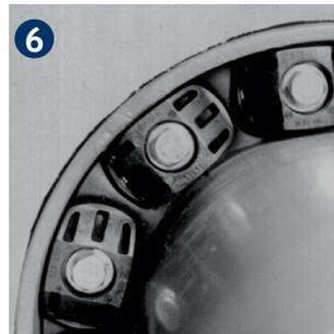
**6** Do not tighten any bolt more than 4 turns at a time. Continue in a clockwise manner. Make 2 or 3 more passes at 3 turns per bolt until links have been uniformly compressed and the max. torque moment (see table) is reached.
